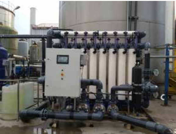
75 m 3 /h Ultrafiltration System
